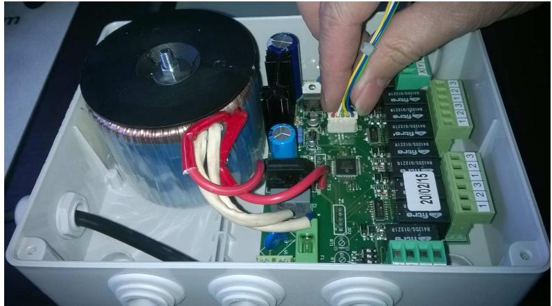
8. Complete the electrical wiring path and make the proper electrical connections by following the wiring diagram on page 13. To facilitate the electrical connections gently remove the electrical junction boxes and then replace them properly.
