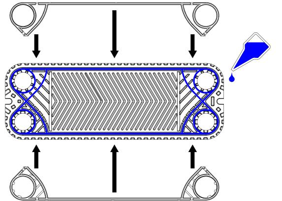
NOTE: In case of heat exchanger with rubber-lined connections, proceed as per below image to seal the initial plate (see fig.5).
